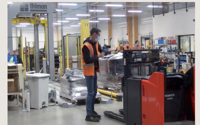
The collector places the pallet in the waiting area and then the packer takes over. This system includes the double-checking of orders, which has halved the number of customer disputes. The automatic plastic-wrapping machine is capable of wrapping 40 pallets an hour and the transparent film is recycled. In total, the Processing Department handles 250 orders every day; from a simple envelope with a nozzle in it, to a full shipping container.
