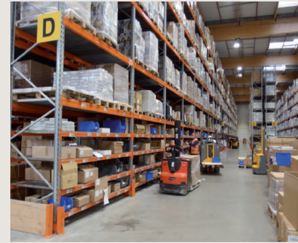
The second storage system consists of storing small products with a high turnover rate on racks in the lower sections. When a collector receives an order, the barcode scanner shows them the location of each part and the easiest and fastest route to its location.
