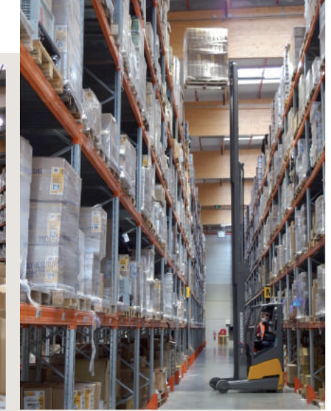
The third storage system used is based on conventional 13-metre high racks (10 metres of which is used). Forklift drivers are in charge of the stacked pallets and they leave them at ground level for the collectors.
